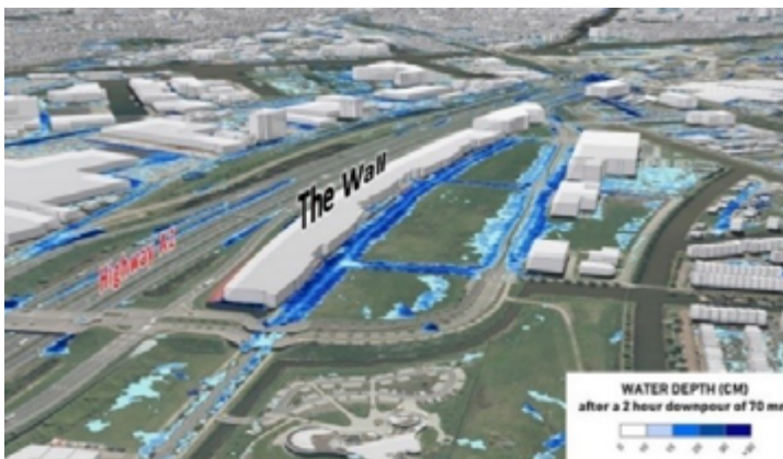
Figure 3. A simulation of the potential flooding following a 2 hour downpour of 70 mm per hour shows that the main access roads to The Wall and part of the A2 highway can be flooded and be inaccessible. Inundation depth is estimated between 20 - 30 cm, potentially damaging the buildings foundation, grid infrastructure or sewer systems, depending on threshold heights of the construction. Source: ClimINVEST, 2019; KNMI, 2014.
